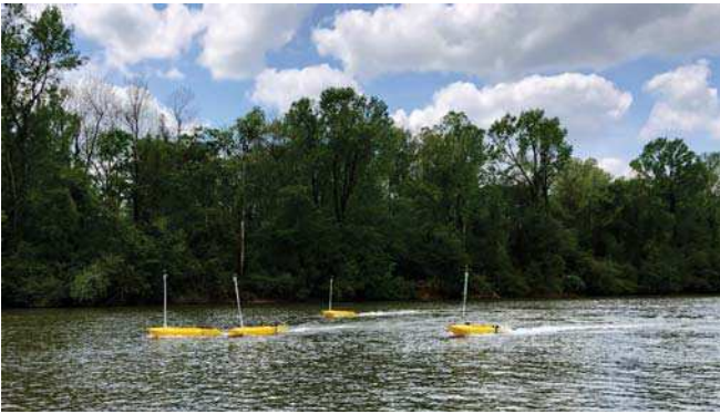
Figure 8. Four Jetyaks operating autonomously in the Congaree River near Columbia, SC.
