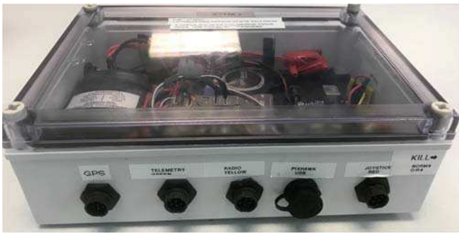
Figure 7. Pixhawk Box with power conditioner, Pixhawk PX4, Arduino Uno, GPS, joystick outputs, remote control interface, MAVLink -MAVROS node proxy inputs/outputs collocated.
