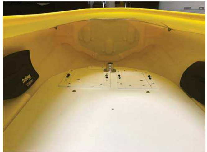
Figure 3. Front portion of marine grade starboard sub-floor with footings for battery, control box, as well as topside and anchor mast ports installed.
